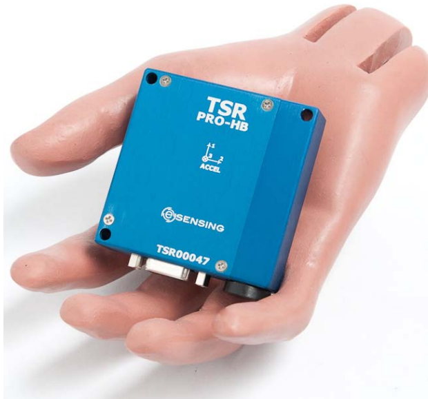
The TSR (65 x 65 x 18 mm) features a triaxial accelerometer and the ability to record up to 20k samples per second per channel.
